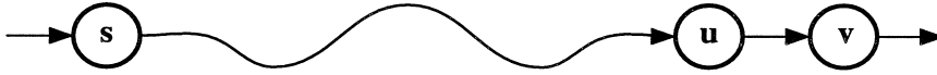
Figure 7: Generation of ill-formed circuits by modified version of the Leiserson-Saxe retiming algorithm. When d(s \stackrel{p_1}{\rightsquigarrow} u) > c for a given clock period c and d(s \stackrel{p_2}{\rightsquigarrow} v) \leq c , then the algorithm results in a negative register count on the edge u \rightarrow v in the retimed circuit.
