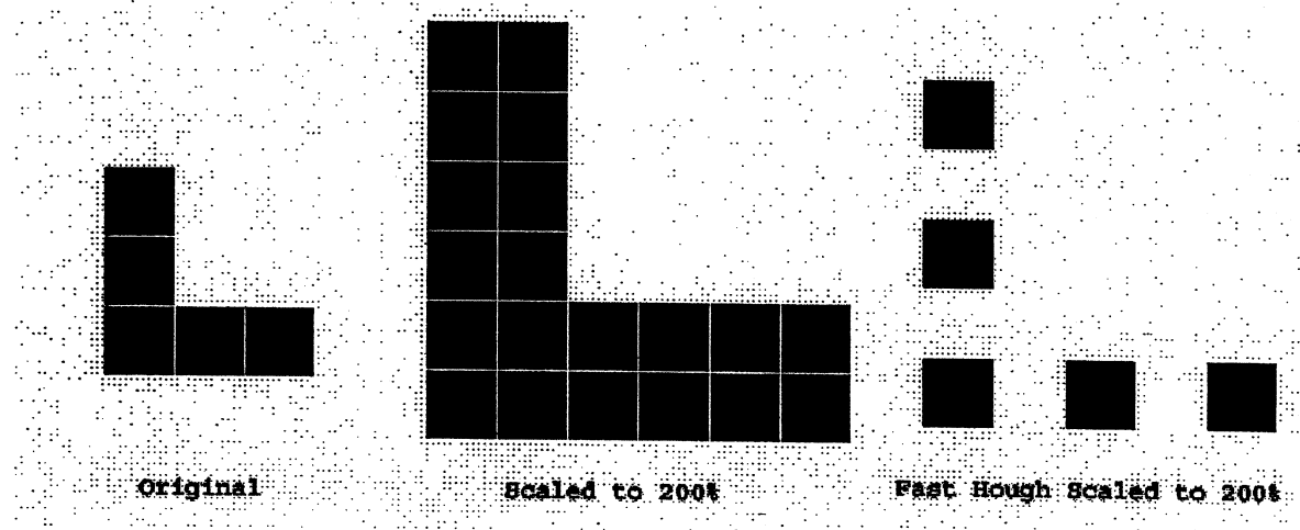
Figure 7. Fast Hough Transform example
