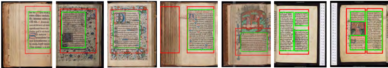
Fig. 7. Block computation results for several example page images, which are respectively from BeineckeMS10 , BeineckeMS109 , BeineckeMS310 , BeineckeMS360 , Osborna44 and BodleianMSBodley850 (from left to right). The two rightmost images show pages from the BodleianMSBodley850 manuscript. The green and red rectangles show the results before and after text block refinement. Manuscript images courtesy of the Yale University [7, 48, 36, 47, 49] and the Oxford University [39].
